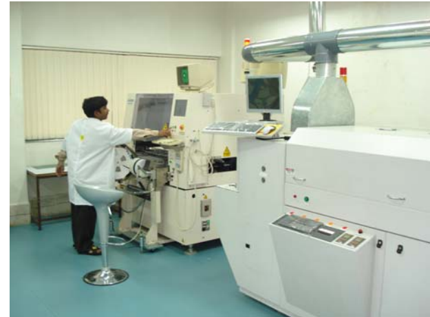
7 Zone Pin & Chain Conveyor Reflow Oven
